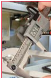
Left: 797 with a DataSure® End Node for wireless data collection Far Left: 797 has IP65 protection against coolant, water, dust and dirt
